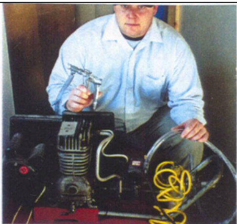
A SMALL COMPRESSOR AND THE QUIKGUN DOES THE JOB @ 80 PSI*
